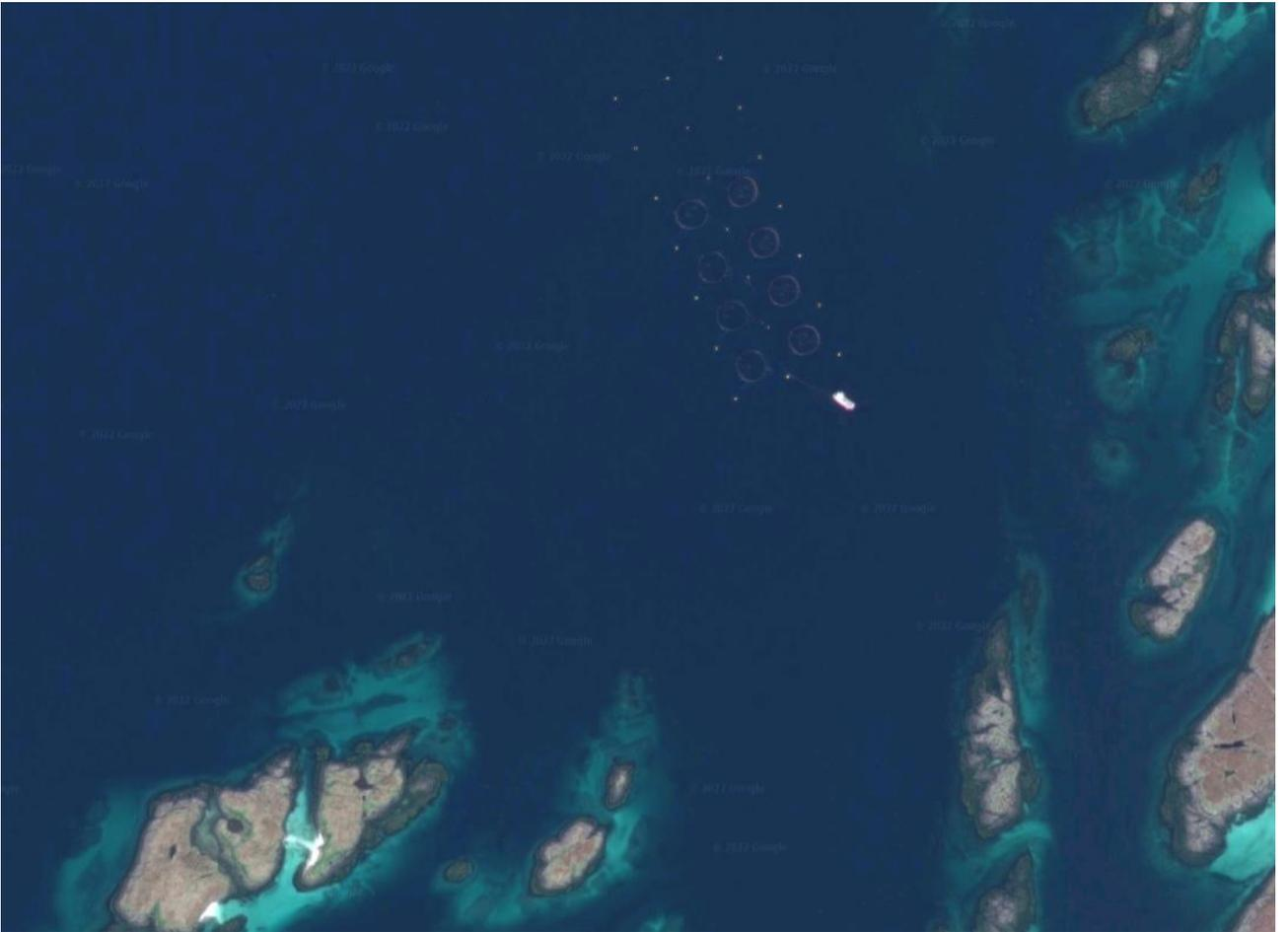
FIGURE 3.31. The facility at Skogsholmen with its eight pen nets and feed barge. *Source: Google*
