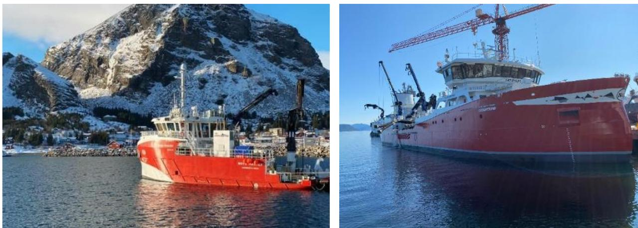
FIGURE 3.15. Examples of ships that might visit the facility. Left: the Nova Master which is used for mooring new facilities. Right: the Færøysund, a well boat used to transport fish. Source: Nova Sea / Marius Vassnes<sup>326</sup>
